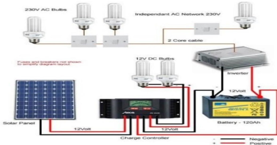
Figure 3: Active Solar Technique
